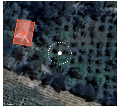
(c) Scene match: the reported GPS coordinate and building footprint are the only geometries in the bounding box of the highest-resolution satellite tile.
